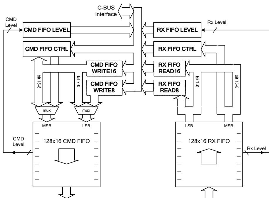
Figure 24 Command and Rx Data FIFOs
