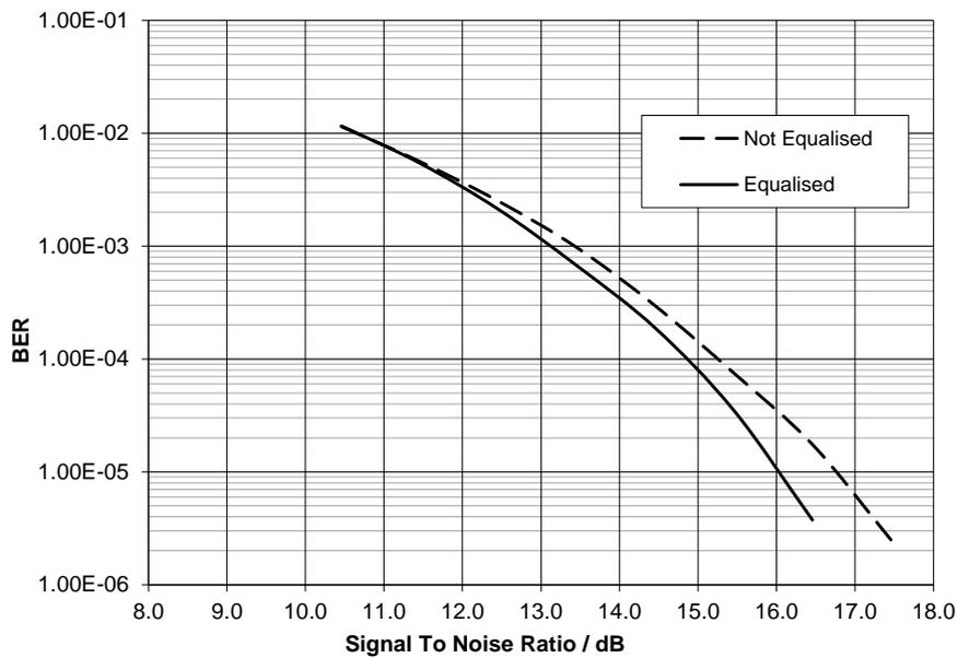
**Figure 47 4-FSK Signal-to-Noise Performance, Equalised and Non-Equalised**
