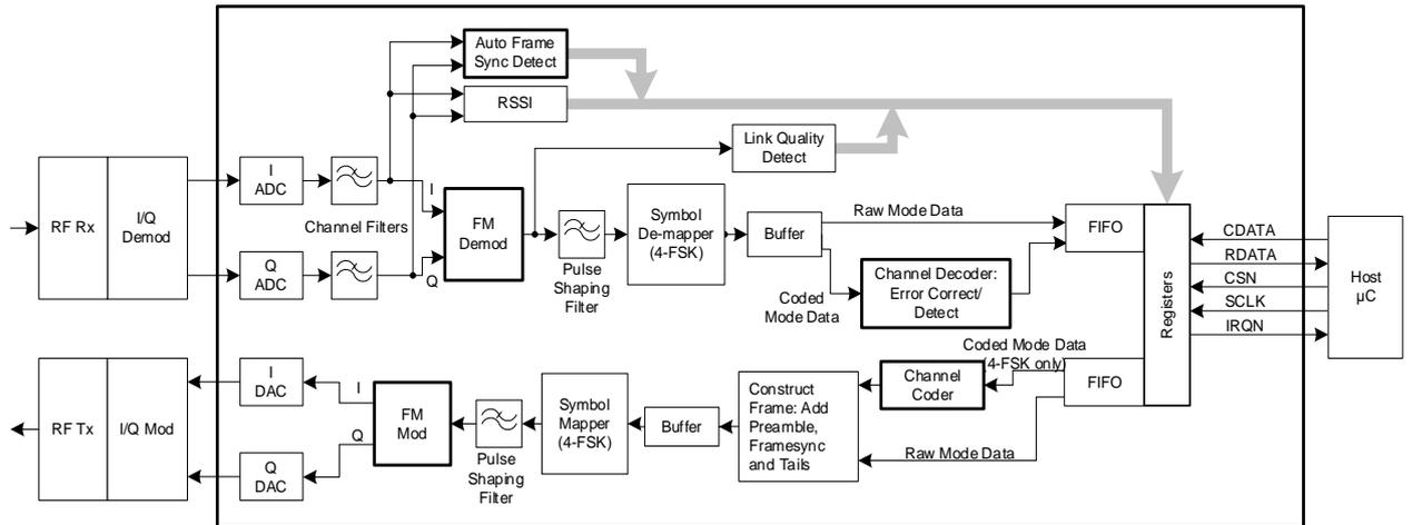
Figure 2 Block Diagram – I/Q Tx and Rx
