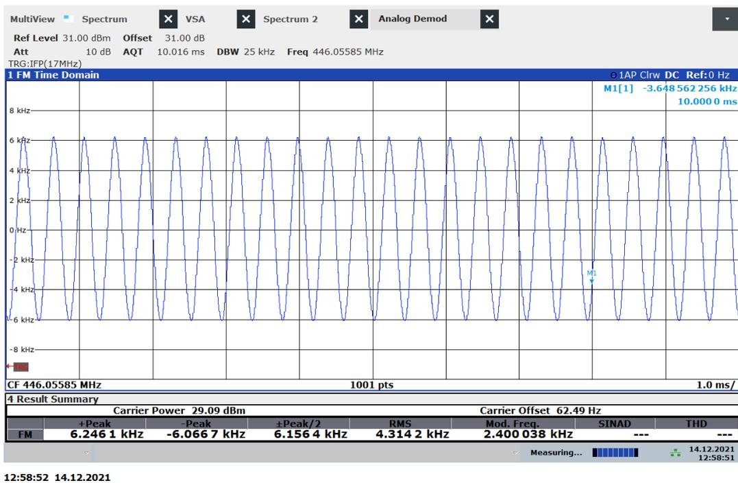
Figure 38 Preamble Pattern for 25kHz I/Q Mode
