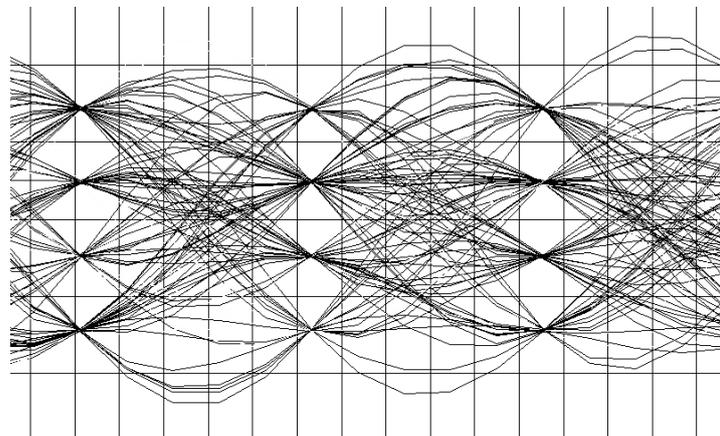
Figure 21 Received Eye Diagram
