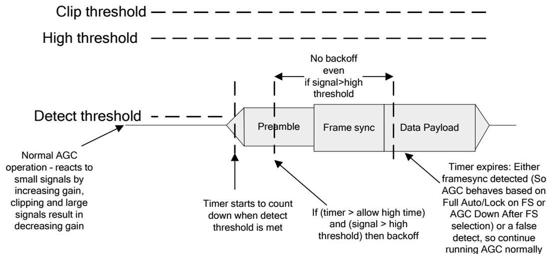
**Figure 27 AGC Behaviour During Burst Reception**
