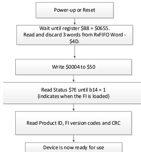
**Figure 14 – Reset without FI Load**
