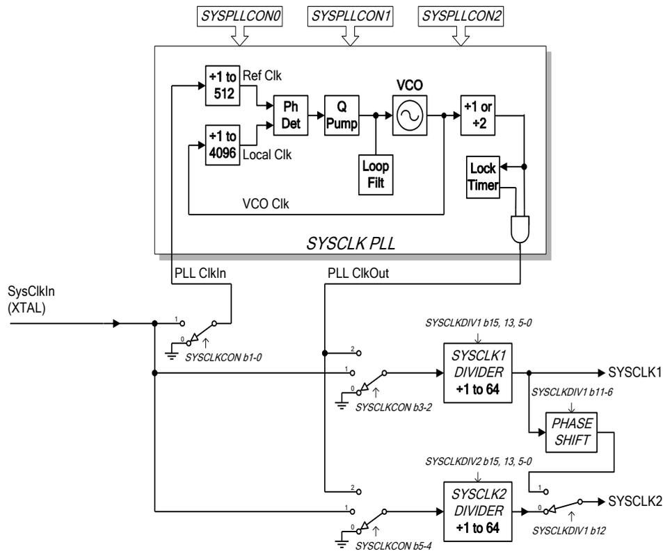
Figure 29 Digital System Clock Generation Schemes
