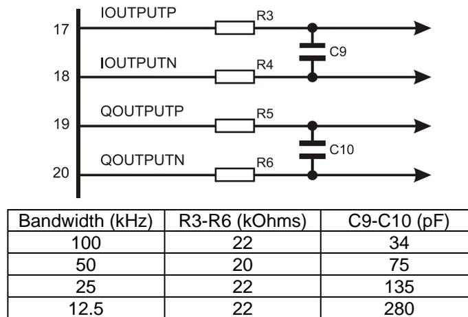
**Figure 7 Recommended External Components – I/Q Output Reconstruction Filter**
