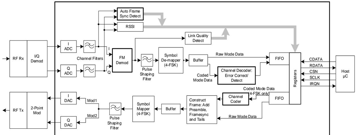
Figure 3 Block Diagram – two-point Tx with I/Q Rx
