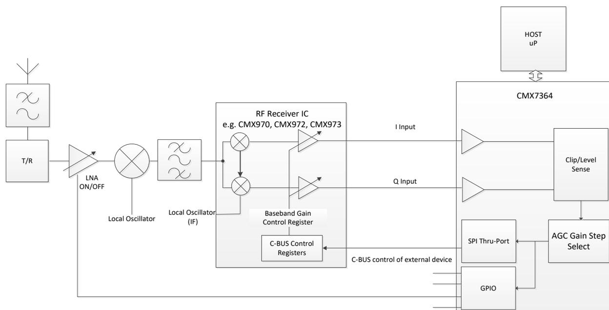
**Figure 26 AGC using SPI Thru-Port and external LNA**
