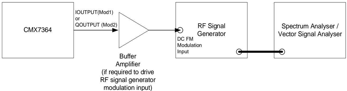
Figure 39 Tx Spectrum and Modulation Measurement Configuration for Two-point Modulation
