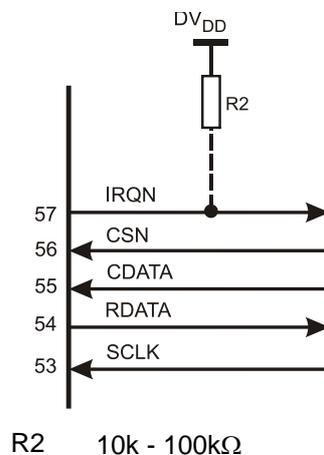
**Figure 6 Recommended External Components – C-BUS Interface**
