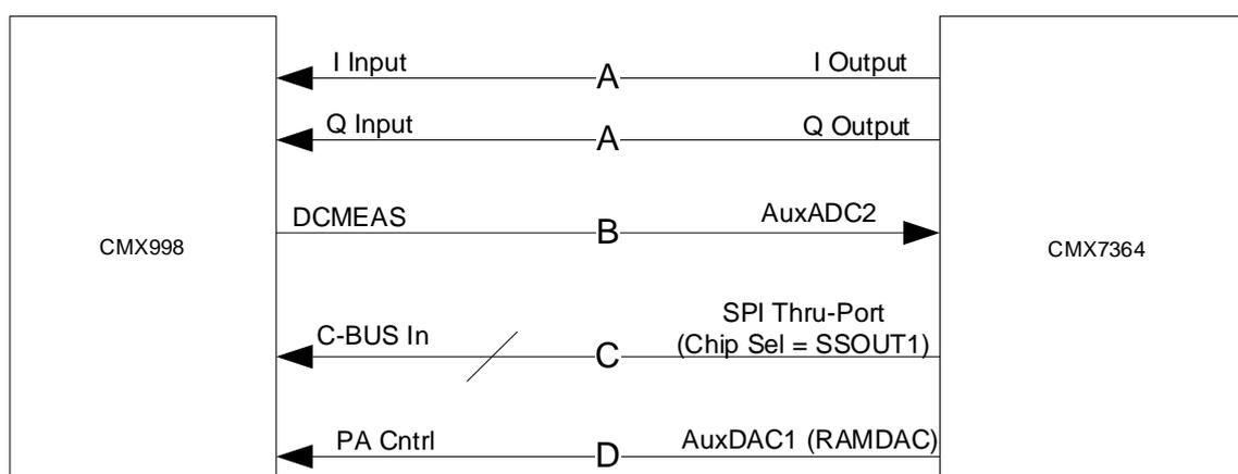
A. The CMX7364 I and Q Outputs are used to provide dc levels, which are adjusted to make the error I/Q measurements equal to the Reference I/Q measurements
