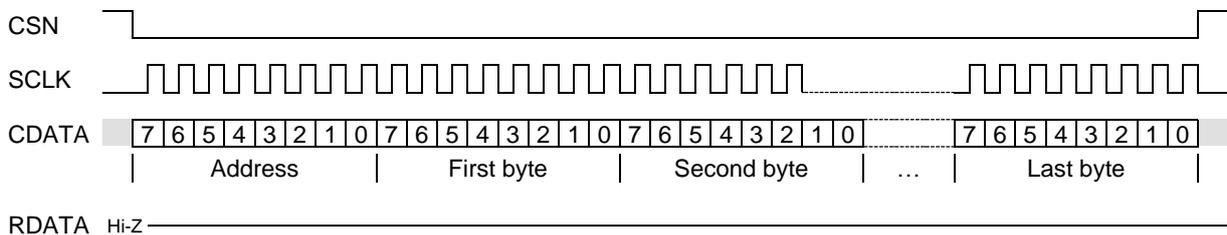
Example of C-BUS data-streaming (8-bit read register)
