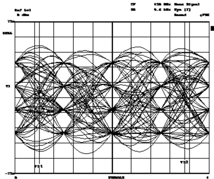
Figure 41 Tx Eye Diagram, 25kHz Two-point Mode
