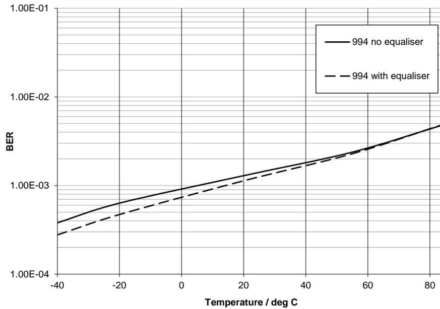
**Figure 48 Performance of Equalised Signals with Temperature Variation**
