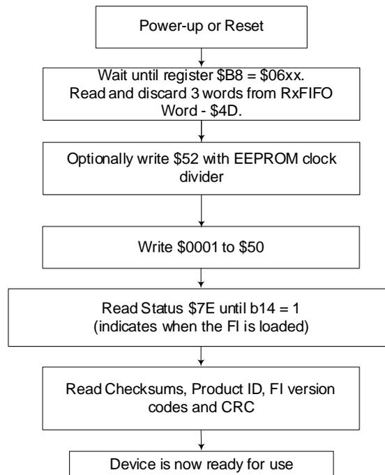
**Figure 13 – FI Loading from Serial Memory**
