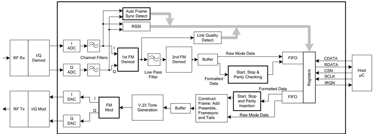
Figure 5 FI-6.x Block Diagram - I/Q Tx and Rx
