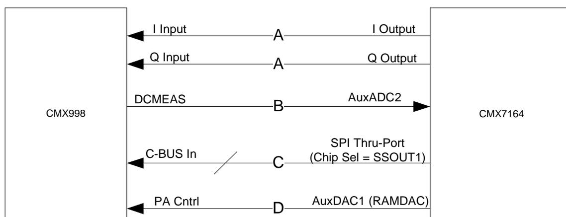
**A. The CMX7164 I and Q Outputs are used to provide dc levels, which are adjusted to make the error I/Q measurements equal to the Reference I/Q measurements**
