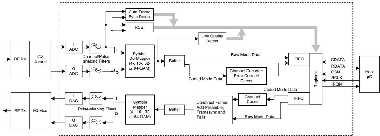
Figure 2 FI-4.x Block Diagram – I/Q Tx and Rx
