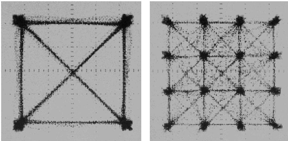
**Figure 86 Received 4 and 16-QAM signals with equalisation**
