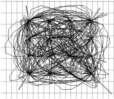
**Figure 25 Constellation Diagram** – no frequency or phase error
