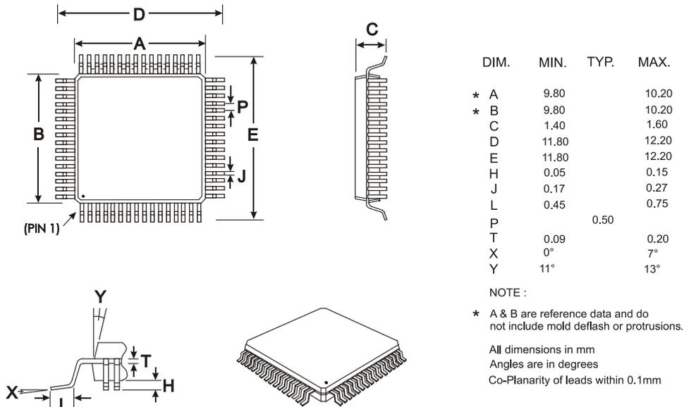
Figure 115 Mechanical Outline of 64-pin LQFP (L9)
