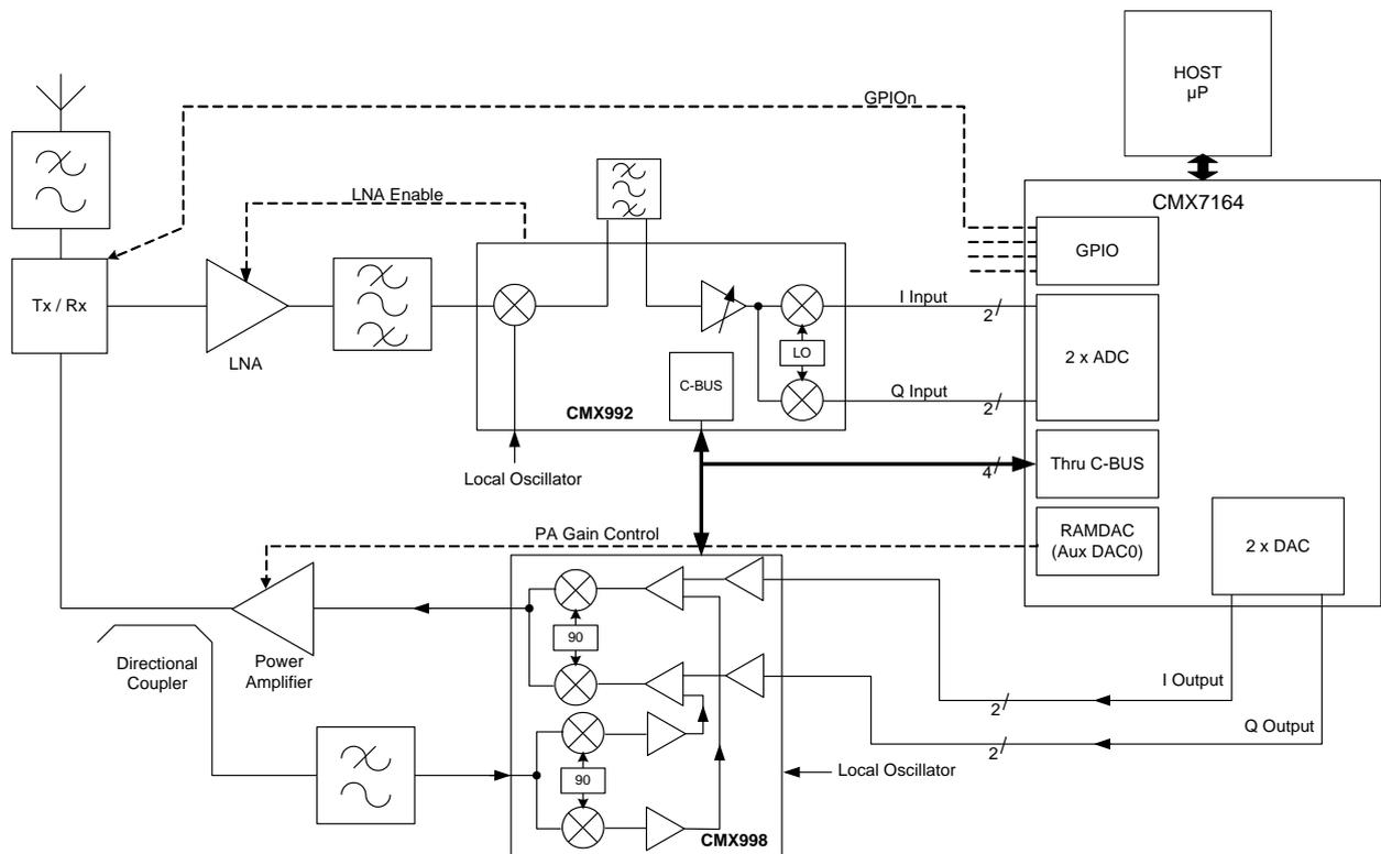
**Figure 44 Outline Radio Design (I/Q in/out for GMSK/GFSK)**
