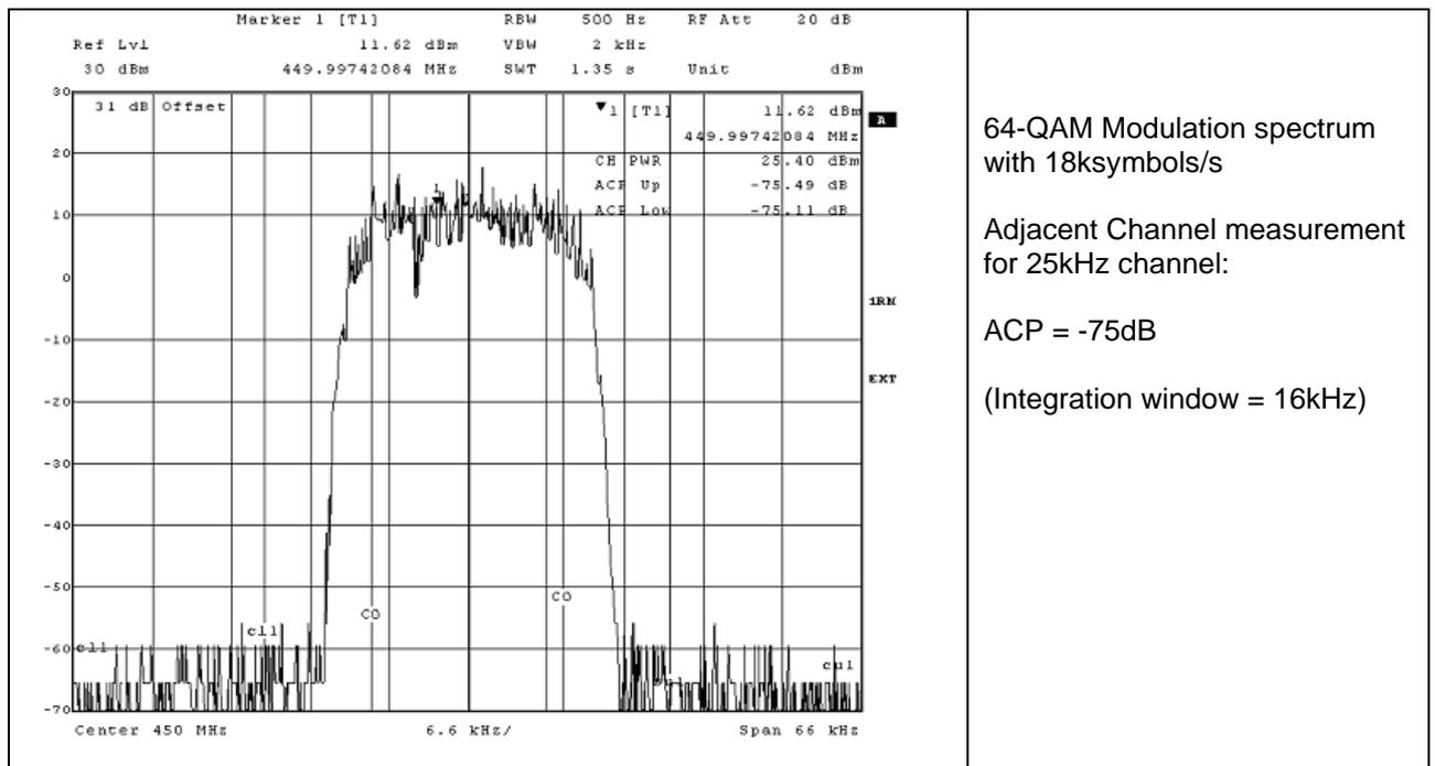
64-QAM Modulation spectrum with 18ksymbols/s
