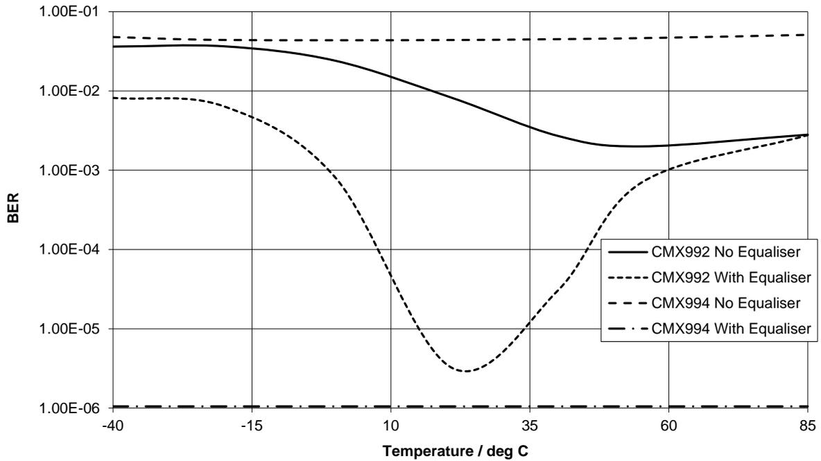
**Figure 106 Performance of 64-QAM Equalised Signals with Temperature Variation**
