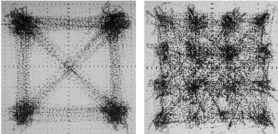
**Figure 85 Received 4 and 16-QAM signals, no equalisation**
