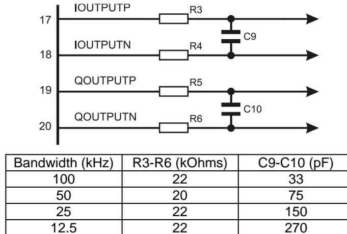
**Figure 10 Recommended External Components – I/Q Output Reconstruction Filter**
