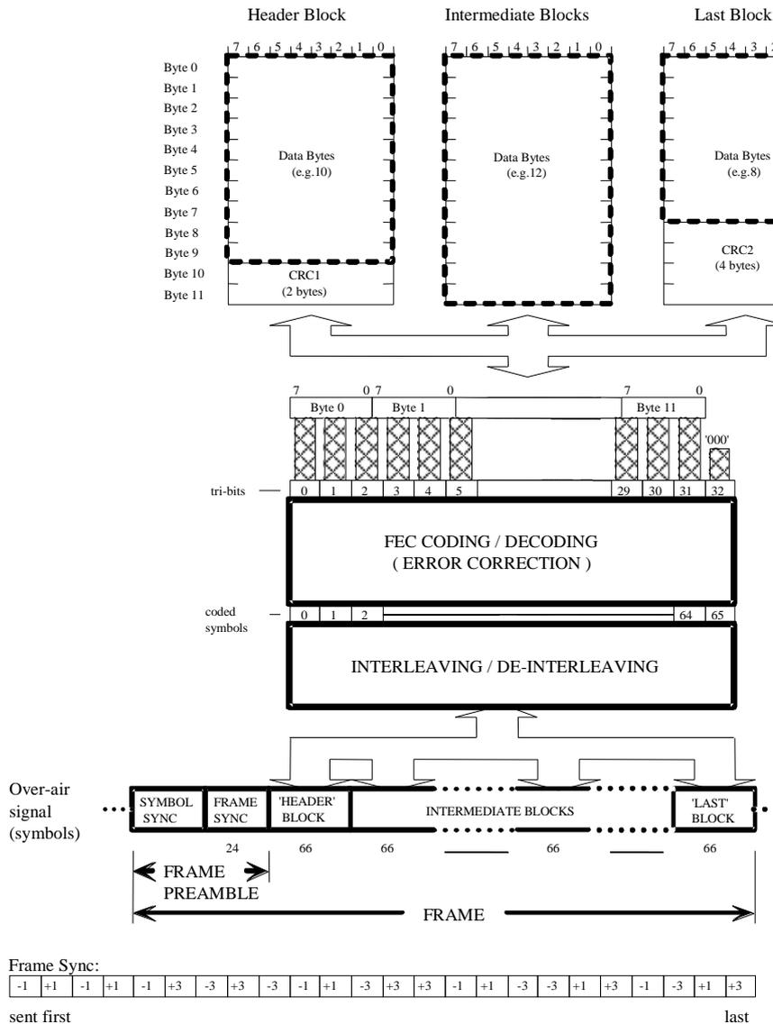
Figure 58 Native Formatted Data Over Air Signal Format
