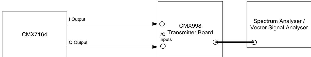
**Figure 87 Tx Spectrum and Modulation Measurement Configuration for I/Q Operation**
