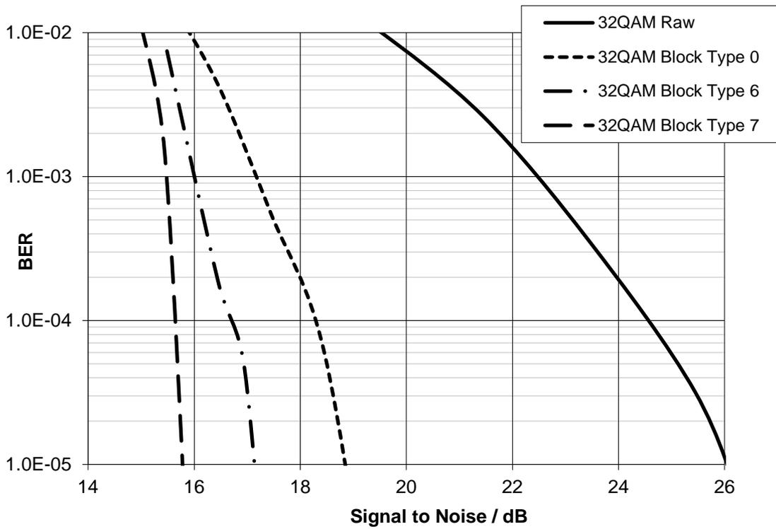
Figure 96 32-QAM Performance with Different Coding Schemes
