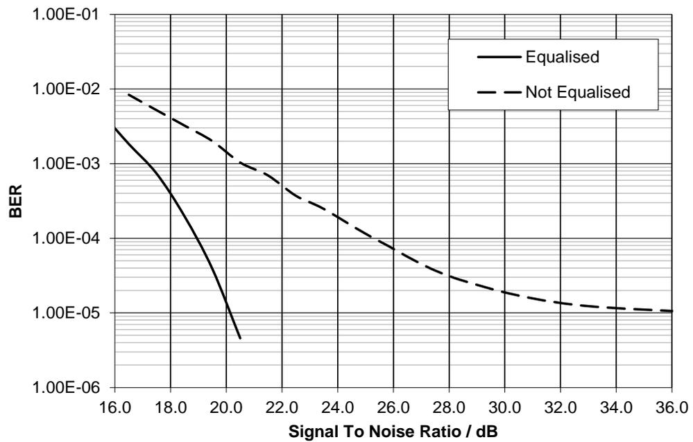
**Figure 103 16-QAM Signal-to-Noise Performance, Equalised and Non-Equalised**
