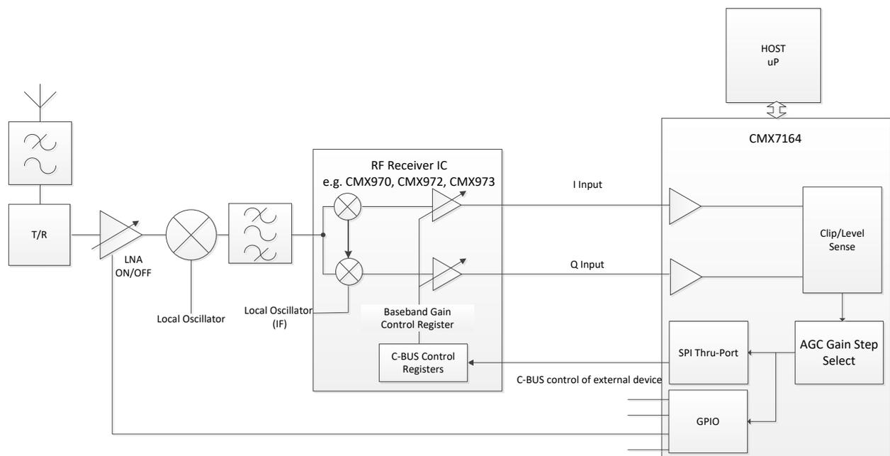
**Figure 40 AGC using SPI Thru-Port and external LNA**
