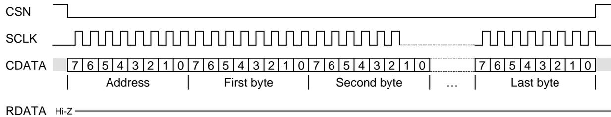
Example of C-BUS data-streaming (8-bit read register)
