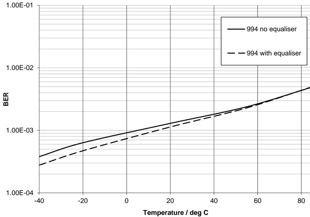
**Figure 81 Performance of Equalised Signals with Temperature Variation**
