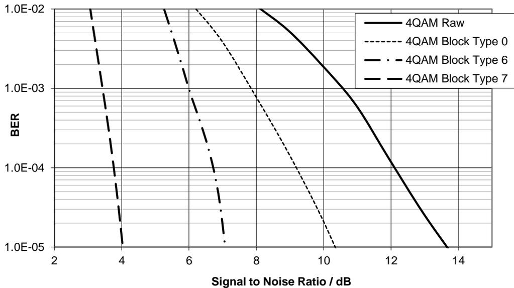
**Figure 94 4-QAM Performance with Different Coding Schemes**
