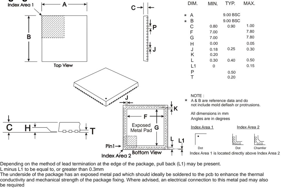
Figure 114 Mechanical Outline of 64-pin VQFN (Q1)
