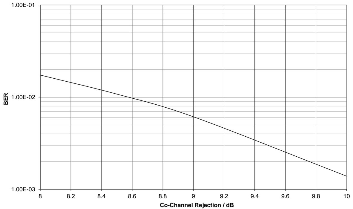
**Figure 71 Modem Co-channel Rejection with FM Interferer (as EN 300 113)**
