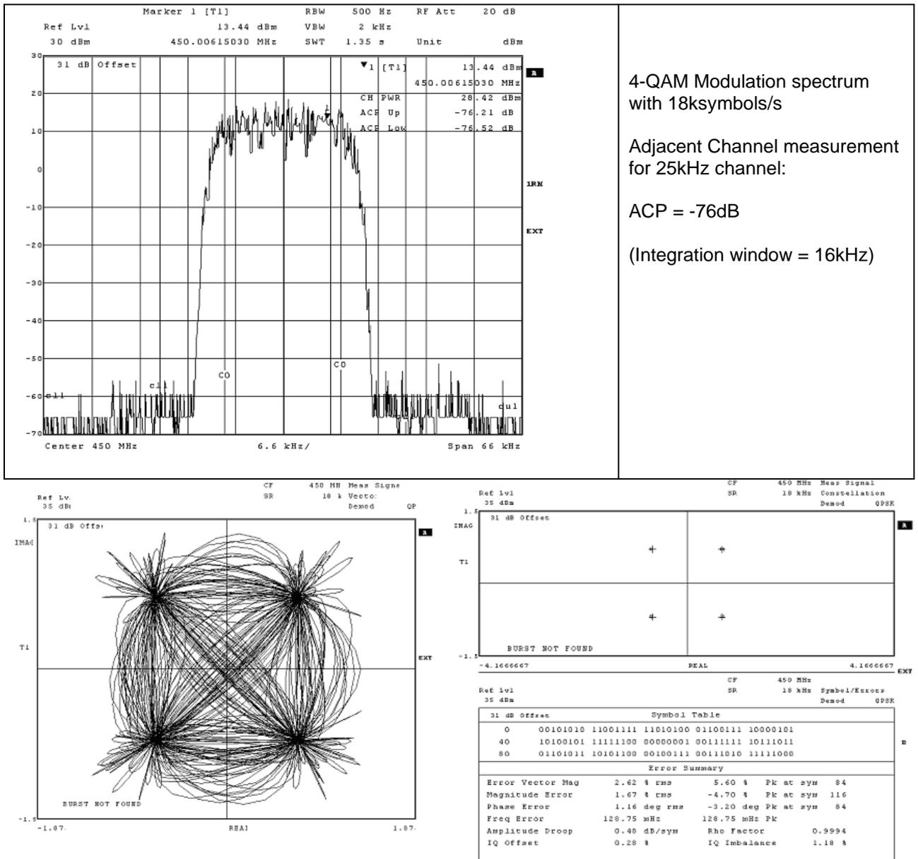
Figure 88 Tx Modulation Spectra (4-QAM), 18ksymbols/s I/Q Modulation into CMX998
