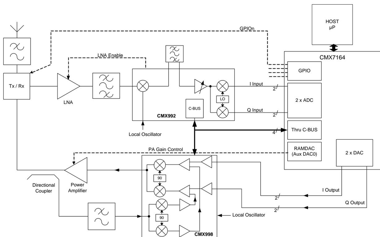
**Figure 83 Outline Radio Design (I/Q in/out for QAM)**
