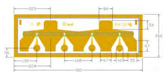
Chip Dimensions: 785 x 260 microns Chip Thickness: 100 microns
