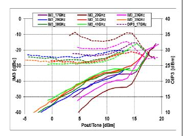
IM3 level [dBc] vs. Input power [dBm/tone]
