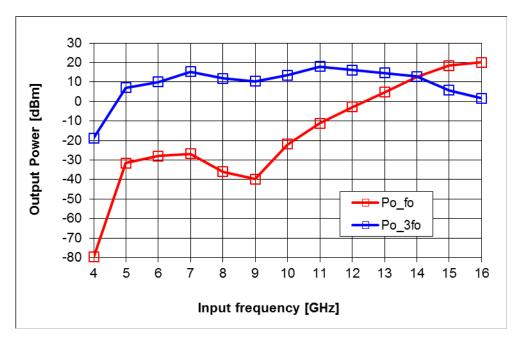
Measured 3x multiplier data: Pin=9dBm, Vd1=1V, Vd2=5V, Vg1=-0.75V, Vg2=-0.75V, Id1=21mA, and Id2=144mA
