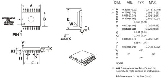
Angles are in degrees Co-Planarity of leads within 0.004" (0.1mm)
